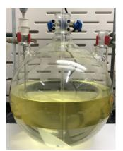
GAPPS on a 100-gram scale in GAP Peptides' lab. Flask size is 12 liters with 4 liters of organic solvent and 3 liters of aqueous wash. Separation is clean and rapid. Scale-up does not require specialized equipment, allows in-process analytics, and reduces process hazards through green chemistry.
